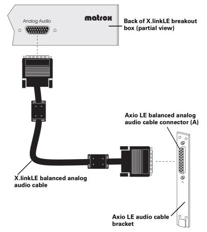
2 Attach the opposite end of the X.linkLE balanced analog audio cable to the balanced analog audio cable connector (labeled A) on your installed Axio LE audio cable bracket. Tighten the thumb screws until snug to ensure a stable connection.
