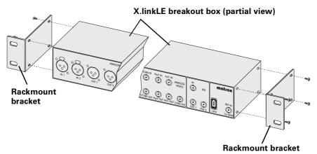
**3** Using a hand screwdriver only (**no power screwdrivers**), carefully tighten each screw until snug. **Do not overtighten**!
