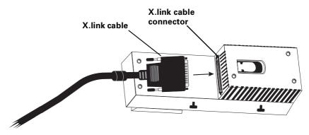
**2** Attach the opposite end of the X.link cable to the bracket connector on the backplate of your installed X.io card.
