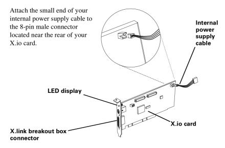
**Note** The connector located between the X.link breakout box connector and the LED display on your X.io card is not used.
