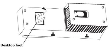
You can use the desktop foot to lay your X.link breakout box flush on your desktop with its audio/video connections facing up. To use the desktop foot, pull the foot out from the back of your breakout box and place the breakout box flush on your desktop.
