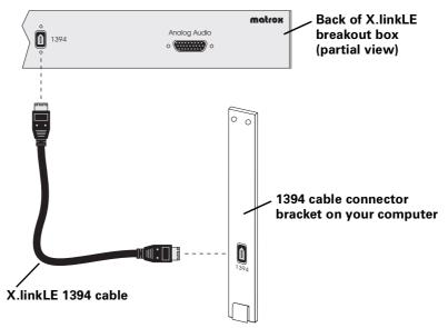
**2** Attach the opposite end of the X.linkLE 1394 cable to the 1394 connector on your computer.
