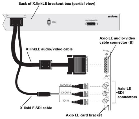
**2** Connect the X.linkLE SDI cable from the back of the X.linkLE breakout box to the respective SDI connectors (labeled OUT A, OUT B, and IN) on your installed Axio LE card.
